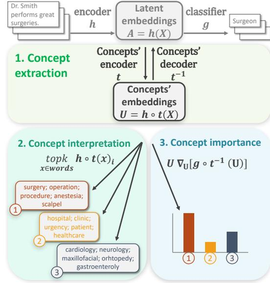
Figure 2: A generalizing formalization of Concept-based explanations. For a model  $f = g \circ h$ , concepts can be extracted from its activations  $A = h(X)$  using the *concept encoder*  $t$ , and can be decoded using the *concept decoder*  $t^{-1}$ . The explanation can be interpreted by keeping the most relevant words for each concept. Finally, an importance score can be attributed to each concept to understand their role in the model’s rationale.
