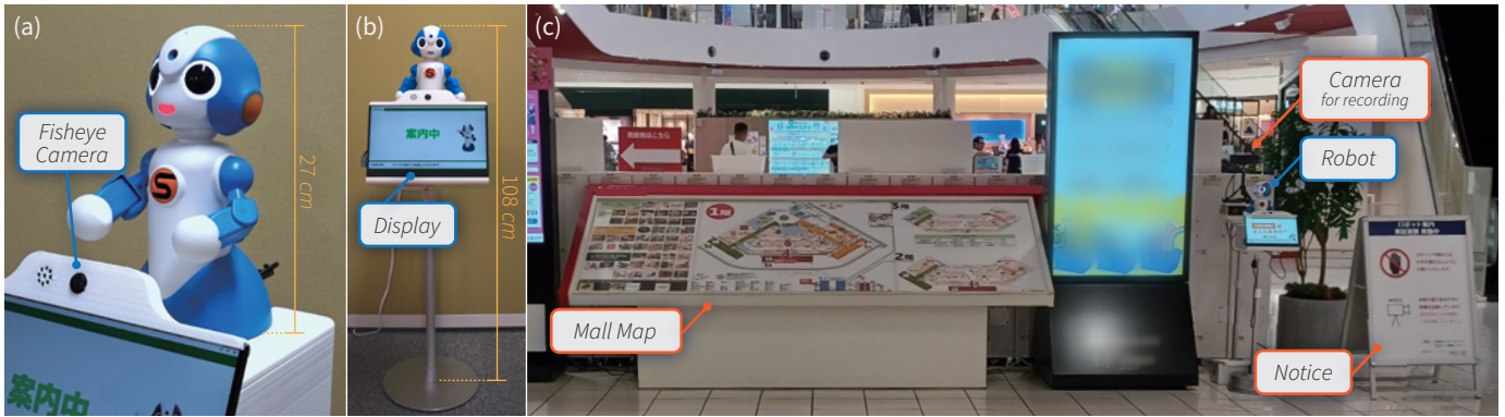
Fig. 2. (a) Sota Robot: The Sota robot, a 27 cm-tall tabletop social humanoid, used in our study, is capable of performing bodily gestures. (b) System Setup: The system consisted of the robot and a display, which complemented the robot’s verbal interactions by showing usage instructions, internal states, and route guidance. (c) Study Setting: The system was deployed on the ground floor of a shopping mall, positioned next to a mall map. A video camera was installed behind the robot, and an experimental notice was placed beside the system.
