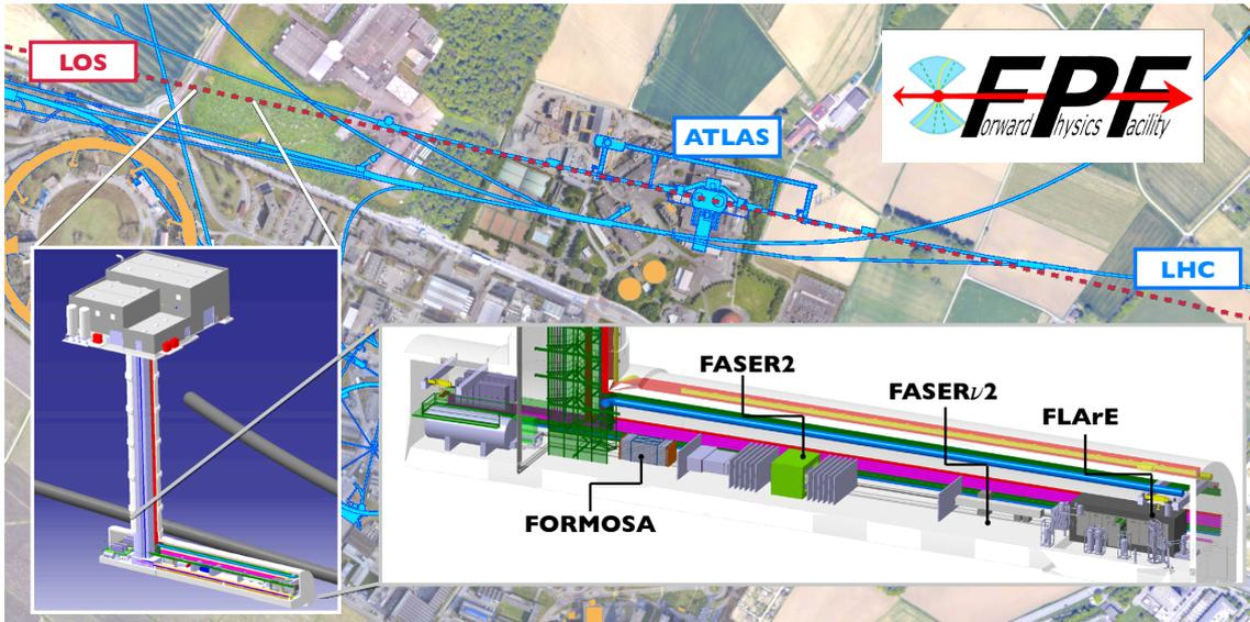
Figure 2: The FPF is located 627–702 m west of the ATLAS interaction point along the line-of-sight (LOS) [3, 4]. The FPF cavern is 75 m long and 12 m wide and will house a diverse set of experiments to fully explore physics in the forward region (see text for details).
