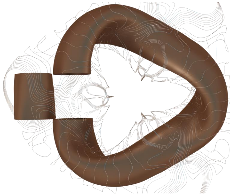
Fig. 5. Plan view of a monolithic blanket toroid, the coil geometry and a 'cut' portion of blanket toroid (length 9 m), which is moved radially. The portion of blanket represents a possible large blanket module still to be developed.
