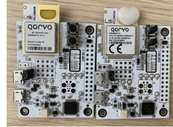
Figure 7: UWB boards with and without glued antenna
