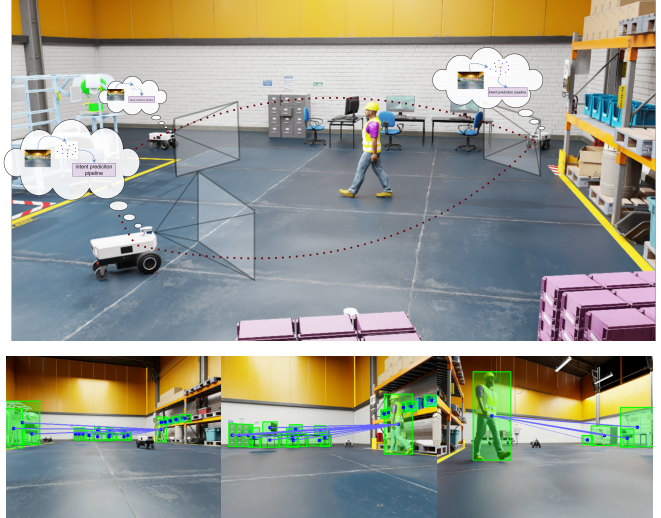
Fig. 1: Overview of the multi-robot system deployed in Isaac Sim for human intent prediction. Robots generate spatial graph representations, integrate neighbor information, employ RNNs for temporal understanding, and converge using a swarm-intelligence-inspired consensus mechanism
