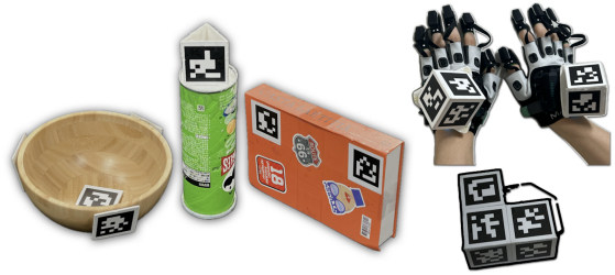
Fig. 4: Objects used in the experiment and a marker system for 3D tracking.
