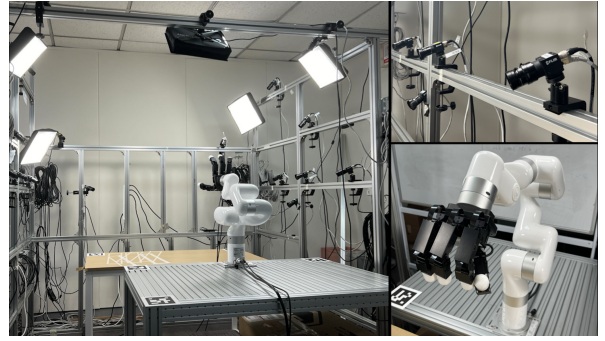
Fig. 3: System Overview: Our system consists of 16 synchronized cameras, an xArm6 robot arm, and a 16-DoF Allegro robot hand.
