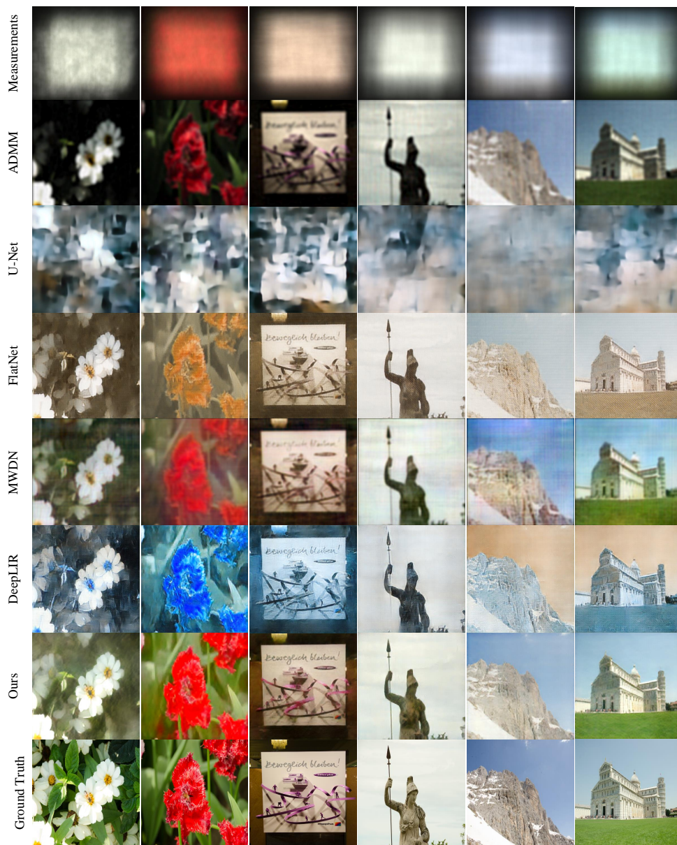
Fig. 3. The test set results for the simulated dataset, from top to bottom, are the Measurements, ADMM, U-Net, FlatNet, MWDN, DeepLIR, Ours, and Ground Truth.
