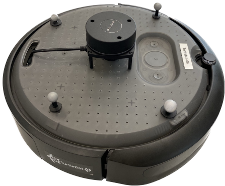
Fig. 8: TurtleBot 4 Lite robot with 2D lidar used for the real-world experimental evaluation.
