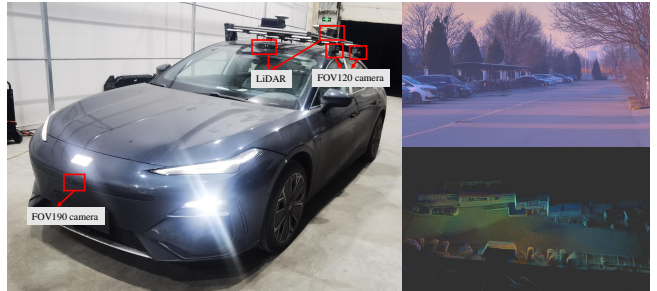
Fig. 6. The self-driving vehicle is fitted with 4 solid-state LiDARs, 10 cameras, with high-precision inertial guidance, and this dataset is collected while in the park.
