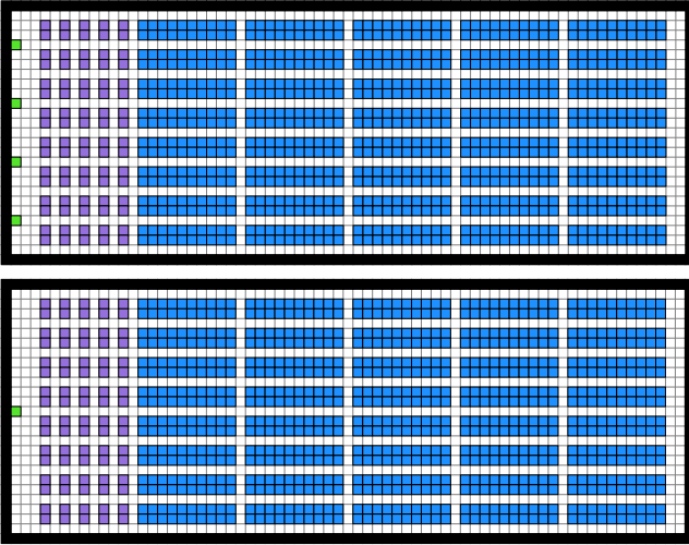
Fig. 1: Warehouse maps: (1) Blue grids represent shelves S . (2) Purple grids represent caches C . (3) Green grids represent unloading ports U . The upper map has multiple ports, while a single port is in the bottom one. In the multi-port map, each unloading port is associated with its own independent cache area, task queue, and set of agents. The cache areas are located near the unloading ports, within a range of \pm 2 rows. In contrast, the single-port map allows the port to utilize all available agents and caches. Given that the number of cache grids can influence the cache hit rate, we tested different configurations by varying the number of cache grids from 80 to 16. This was achieved by progressively removing cache grids column by column from right to left.
