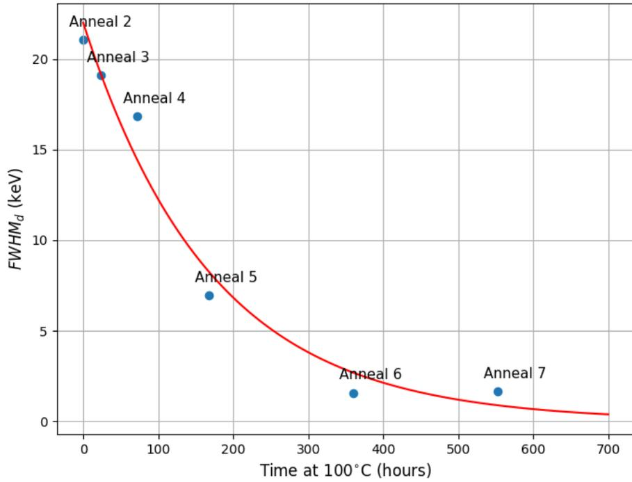
Figure 5:  $FWHM_d$  (component due to radiation damage) plotted against time spent annealing at  $100^\circ\text{C}$ , for hole-collecting strips utilizing a Cs-137 source. An exponential decay function is fit to the datapoints and plotted in red. We find the best fit when  $FWHM_{d,0} = 22.01 \pm 1.2 \text{ keV}$  and  $\tau = 171 \pm 26$  hours.
