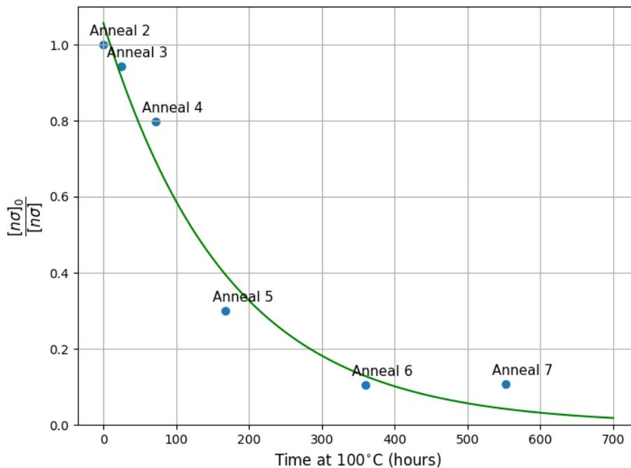
Figure 6: Decay of post-radiation trap density over time spent annealing at 100°C. The y-axis tracks the decrease in trap density (and increase in trapping product) by dividing the post-anneal 2 trapping product  $[n\sigma]_0^{-1} = 93 \text{ cm}$  by the trapping product measured each successive anneal  $[n\sigma]^{-1}$ . An exponential decay function is fit to the data points and plotted in green. We find the best fit when  $[\frac{n}{n_0}]_0 = 1.06 \pm 0.06$  and  $\tau = 170 \pm 29$  hours.
