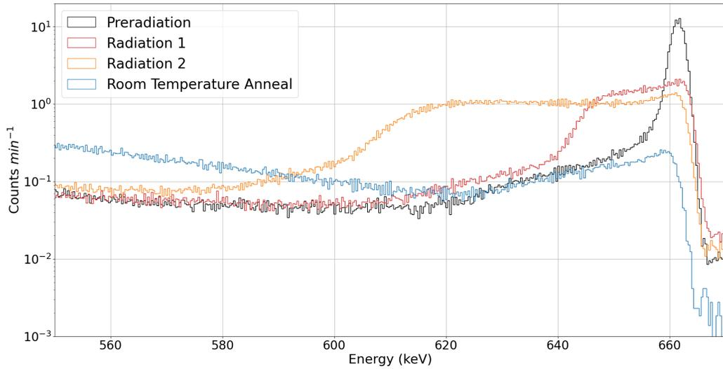
Figure 2: Counts per minute of hole-collecting strips for Cs-137 source plotted on a logarithmic scale. Counts collected: prior to radiation or annealing (black), after receiving  $2.00 \times 10^8 \text{ p}^+/\text{cm}^2$  (red), after receiving a total  $4.95 \times 10^8 \text{ p}^+/\text{cm}^2$  (orange), and after annealing at room temperature for 14 days (blue).
