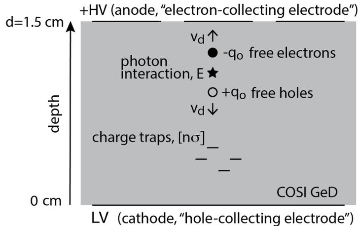
Figure 1: Charge transport in COSI GeDs
