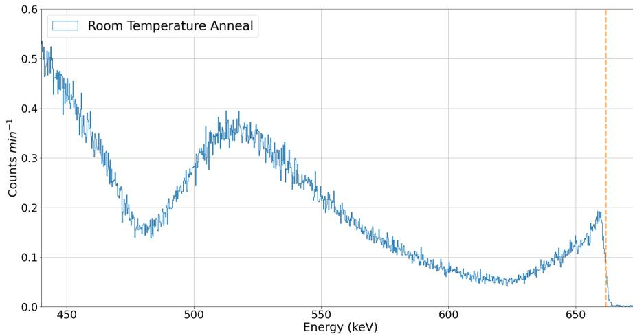
Figure 3: Counts per minute of hole-collecting strips for a Cs-137 source after annealing at room temperature for 336 hours. An orange dashed line marks 0.662 MeV, the decay energy of Cs-137.
