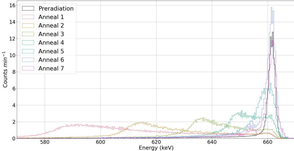
Figure 4: Counts per minute for hole-collecting strips for a Cs-137 source across incremental high-temperature anneals. Anneals and their respective FWHM measurements are listed in Table 2.
