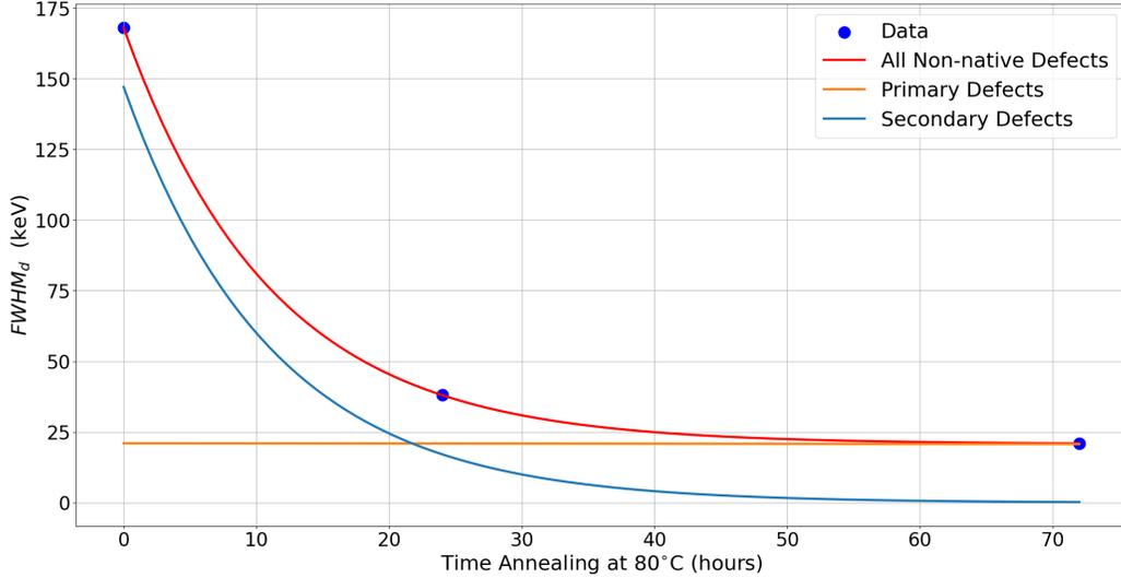
Figure 7: Anneals at 80° fitted by a double exponential function plotted in red. Decay for primary defects, assuming  $\tau_1 \gg 72$  hours, is plotted in orange, while decay for secondary defects is plotted in blue.
