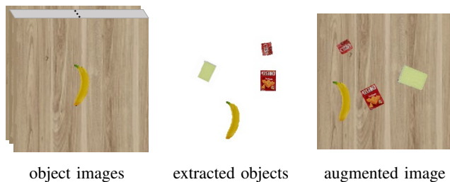
Fig. 7: Object-level data augmentation. We extract objects from the images of a single object, apply the augmentation methods (e.g., shifting, rotation), and assemble them on a background to generate diverse adaptation data for adversarial adaptation.
