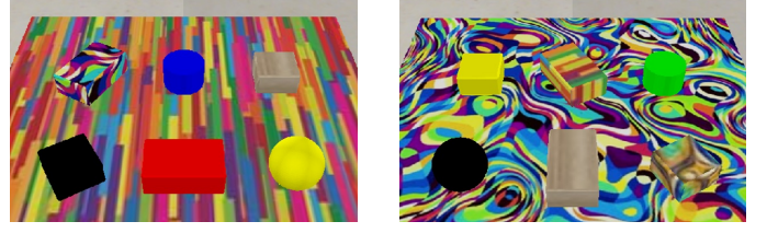
Fig. 4: Examples of basic objects. Synthetic objects of various colors and shapes are used for learning object attributes and grasping affordances. To ensure shape attribute learning, we include objects having random textures.
