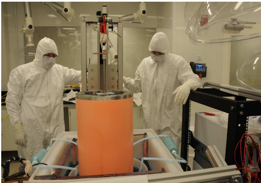
FIG. 3. A mandrel with copper undergoing inspection at the PNNL Shallow Underground Laboratory.
