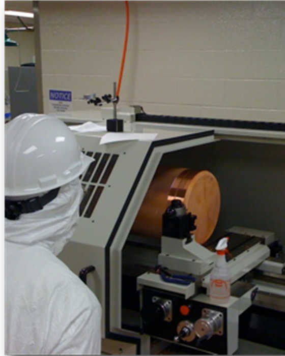
FIG. 6. EFCu on mandrel being machined on the large TRAK lathe in the underground machine shop.
