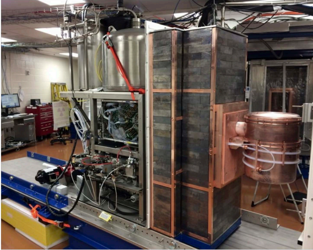
FIG. 36. A shield monolith in transit with cryogenic services, shielding, module and calibration track.
