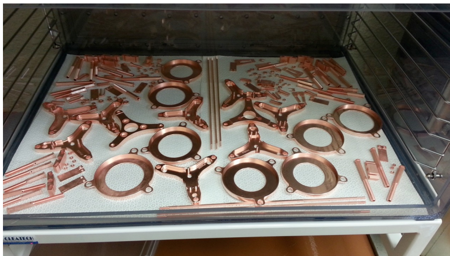
FIG. 8. A selection of small copper parts fabricated in the underground machine shop.
