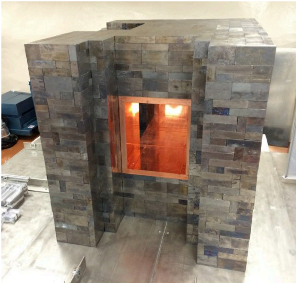
FIG. 35. The DEMONSTRATOR outer copper and lead shield showing the keyed openings for the monoliths. Only the outer copper shield was installed when this photograph was taken.
