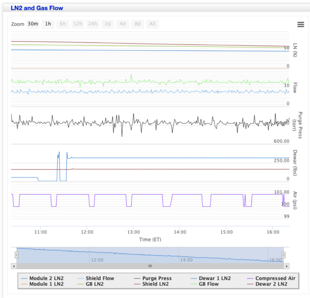
FIG. 40. A screenshot, taken on 11/7/22, of a part of the passive web-based monitoring tool developed for the DEMONSTRATOR. Descriptions of the different traces are provided at the bottom of the figure.
