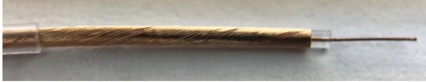
FIG. 26. Example of the high quality strip-back obtained using the CoaxStrip Machine
