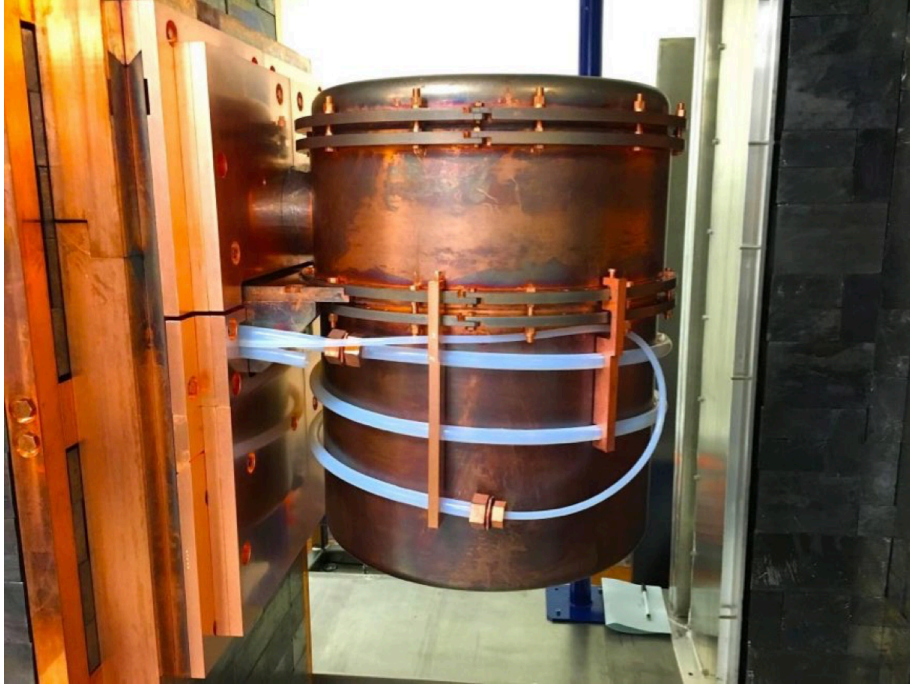
FIG. 33. Picture of helical PTFE calibration track mounted around a module. The thinner tube was for the nitrogen purge.
