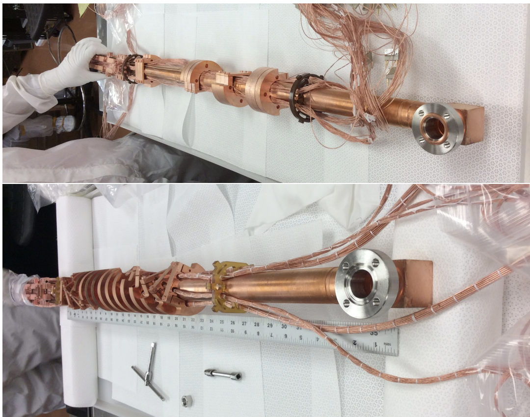
FIG. 27. (Top) The original baffle plate arrangement on the thermosyphon with 12 baffle plates, split into 4 groups of 3 at orthogonal angles. Cables were not bundled. (Bottom) The new baffle plate arrangement after the upgrade with 16 baffle plates, each plate at a staggered angle from the previous plate. Cables were bundled with plain dental floss per NASA specifications.
