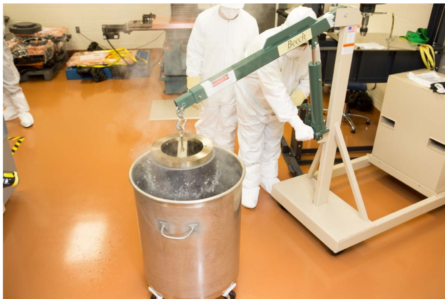
FIG. 7. Copper being removed from mandrel via thermal shock.
