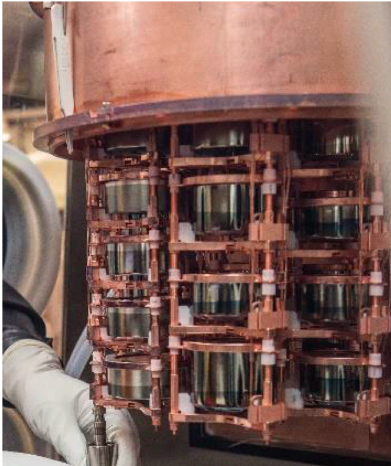
FIG. 19. Module 1 with loaded strings inside glovebox and prior to closure of the Module 1 cryostat and IR shield.
