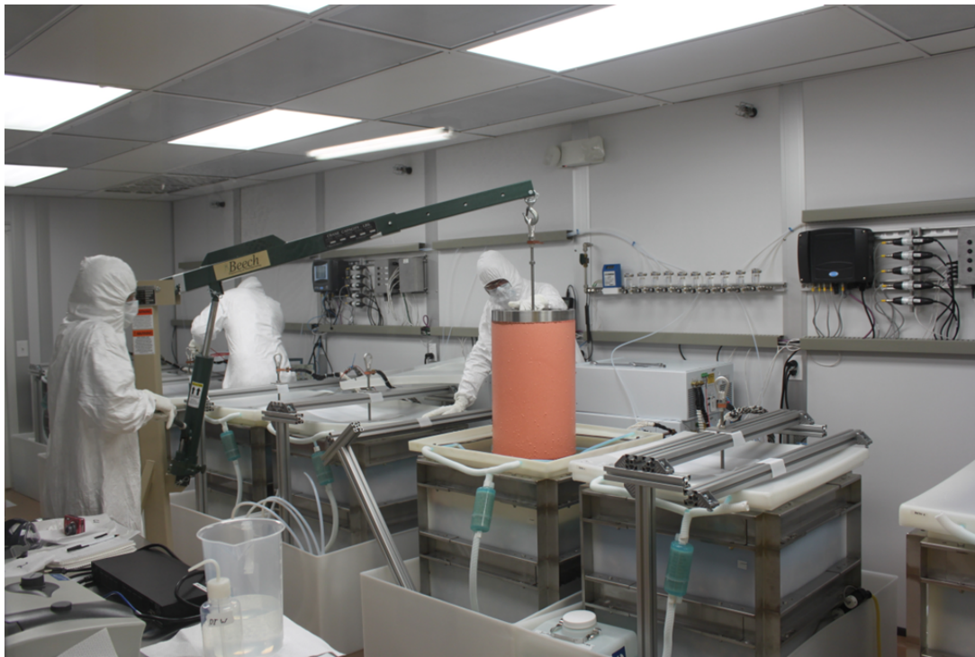
FIG. 5. A copper coated mandrel being inspected over its electroforming bath in the temporary cleanroom.
