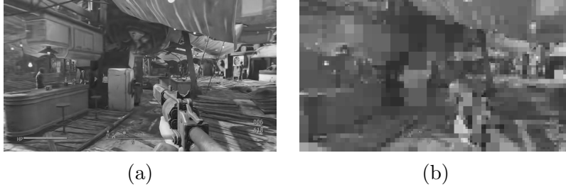
Figure 4: (a) The original decoded frame in grayscale (b) The partition map of the frame
