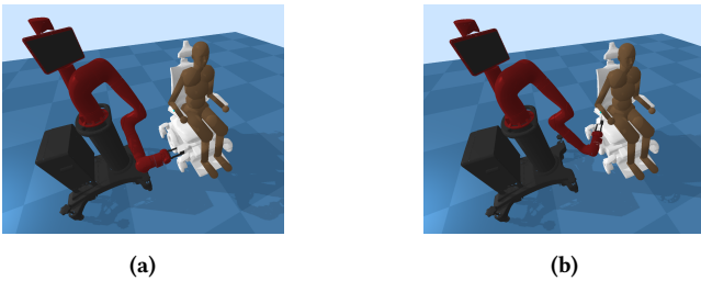
Figure 5: Initial and goal positions in the ScratchItchSawyer environment from AssistiveGym. (a) The initial configuration. (b) The goal configuration, where the robot arm is positioned to scratch the target area, close enough to alleviate the itch.
