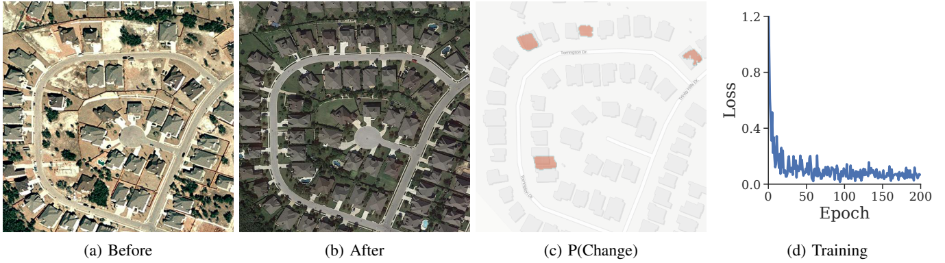
Fig. 5: Neural sensing of geographic change: Before (a) and after (b) images taken by a satellite provide the input for the ChangeFormer, resulting in a prediction of change (c) after training the model on ground-truth data (d). By associating the prediction with points in state-space, it is translated into HPLP clauses as in Listing 3. Note how the ChangeFormer is, on the one hand, not perfect and missed some of the construction sites in the west, but, on the other hand, identified a building that is not part of OpenStreetMaps at the time of writing (center-top).
