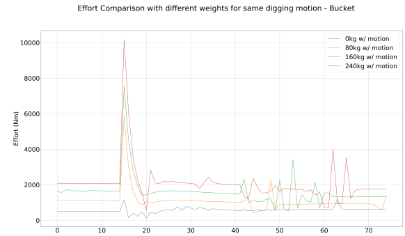
Fig. 7: Effort on Bucket Joint (Simulation)
