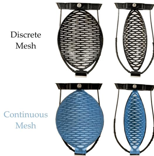
**Figure 4.** Two variations of Kiri-Spoon’s mesh. (Top) For most foods a discrete mesh is sufficient. (Bottom) However, for liquid foods such as soups, a thin membrane can be mounted to the kirigami sheet. The resulting continuous mesh prevents liquids from falling out of the bottom of Kiri-Spoon.
