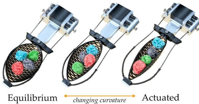
**Figure 2.** Actuating and releasing Kiri-Spoon. The core element of Kiri-Spoon is an elliptical kirigami sheet with discrete ribbons orthogonal to the applied forces. Retracting one end of Kiri-Spoon causes this 2D sheet to buckle and form a 3D bowl with increasing curvature, thereby encapsulating food items.
