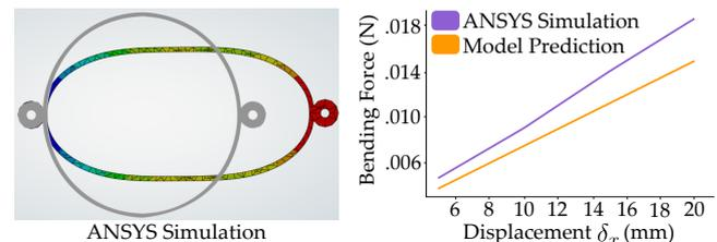
**Figure 14.** Physics simulation in support of Equation (2). (Left) ANSYS simulation environment. The initial circular boundary is shown in grey, while the colored ellipse depicts the deformed elliptical boundary for a displacement of 20 millimeters. (Right) Simulation results showing that the force predicted by our model in Equation (2) is a lower bound on the actual tensile force required to bend the boundary ribbon.
