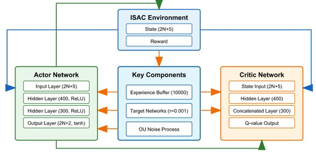
Fig. 1. The framework of DDPG.
