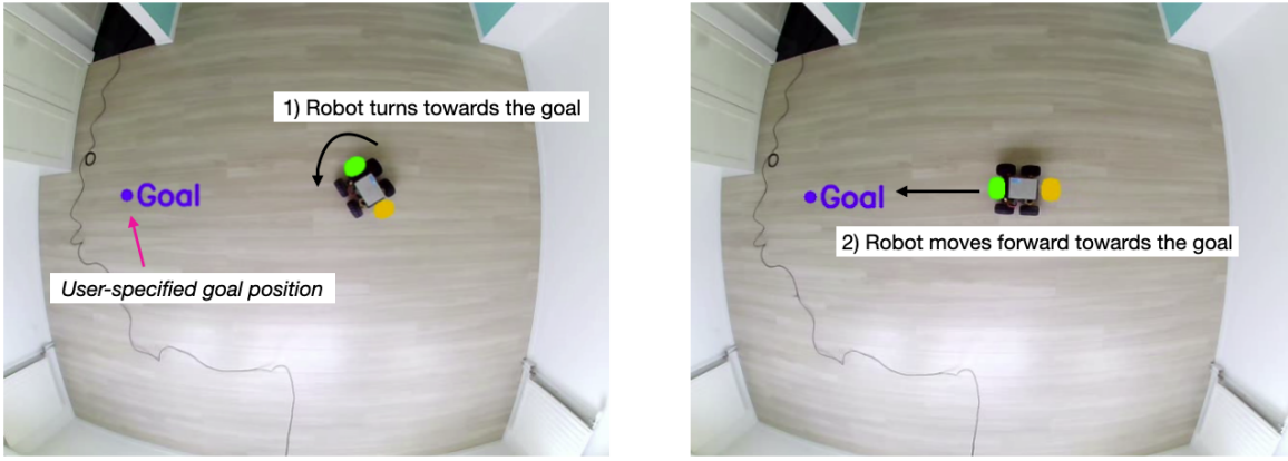
Fig. 6: Experiment 1: Steering the robot towards a user-specified goal. First, the user specifies a goal position to be reached by clicking on the desired location on the image plane. Upon receiving the user-specified location, the python script running the visual positioning algorithm described in Section III computes the real-world goal and robot coordinates, and sends commands to the robot via WIFI (see Fig. 1) in order to steer it towards the user-specified goal location. The steering is done by 1) turning the robot towards the goal position and 2) moving forward until the goal is reached.
