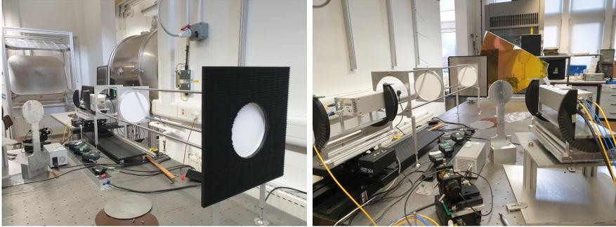
**Fig. 5:** The test setup can be seen (Left) looking towards the receiver from the side of the collimating mirror and (Right) looking towards the collimating mirror from an intermediate angle behind both launcher and receiver.
