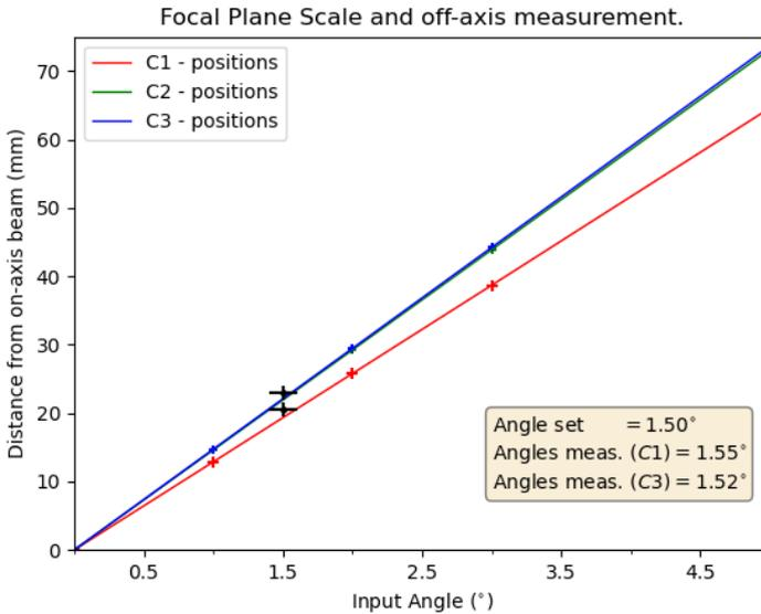
**Fig. 9:** Telescope plate scale estimated for the three configurations compared with the measured case. Measured off-axis focus is shown for two configurations as the black dots with relevant error bars, showing good agreement with the expected focal plane scale.
