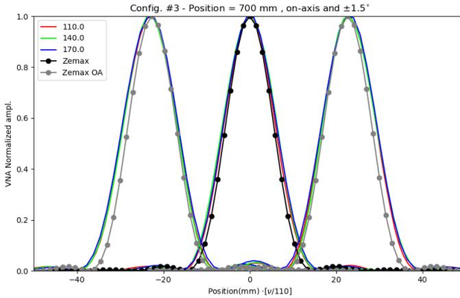
**Fig. 8:** The beam cut comparison performed at frequencies 110,140 and 170 GHz and at angles  $-1.5^\circ, 0^\circ, 1.5^\circ$ . Circle marker-lines show the respective expected on-axis (black) and off-axis (gray) profile from optical ray-tracing simulations.
