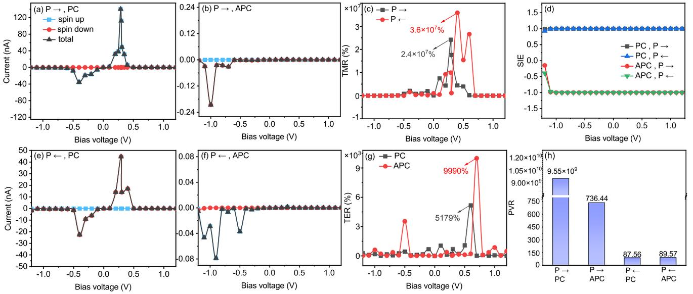
FIG. 4. The variation of the spin current [(a), (b), (e), and (f)], TMR ratio (c), TER ratio (g), and spin injection efficiency (SIE) (d) *vs* the bias voltages and the current peak-to-valley ratio (PVR) (h) in PtTe<sub>2</sub>/CrBr<sub>3</sub>/MnPSe<sub>3</sub>/CrBr<sub>3</sub>/CrBr<sub>3</sub>(Li) MFTJs with different polarization directions and magnetic configurations.
