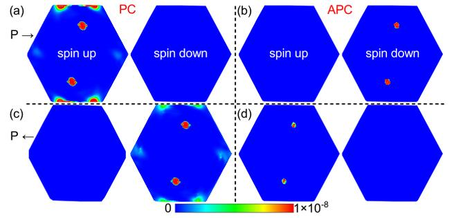
FIG. 3. The  $k_{\parallel}$ -resolved transmission coefficients of  $\text{PtTe}_2/\text{CrBr}_3/\text{MnPSe}_3/\text{CrBr}_3/\text{CrBr}_3(\text{Li})$  MFTJs in the 2D Brillouin zone at the Fermi level for the  $P \rightarrow/P \leftarrow$  and  $PC(M\uparrow\uparrow)/APC(M\uparrow\downarrow)$  states.
