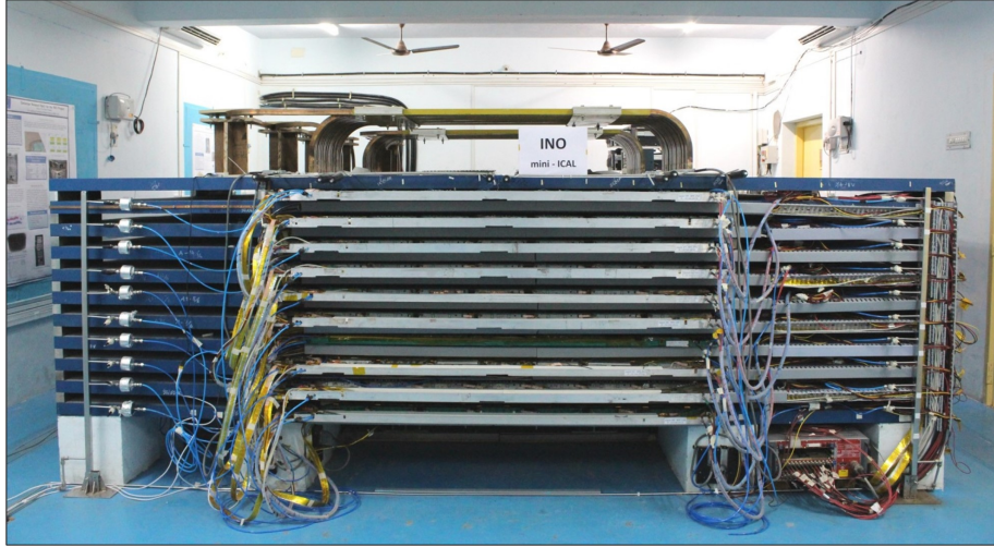
Figure 10: Mini-ICAL Experiment with RPC Detector Units.
