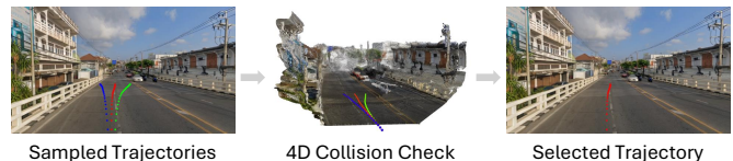
Fig. 9. Demonstration of how DreamDrive helps motion planning.
