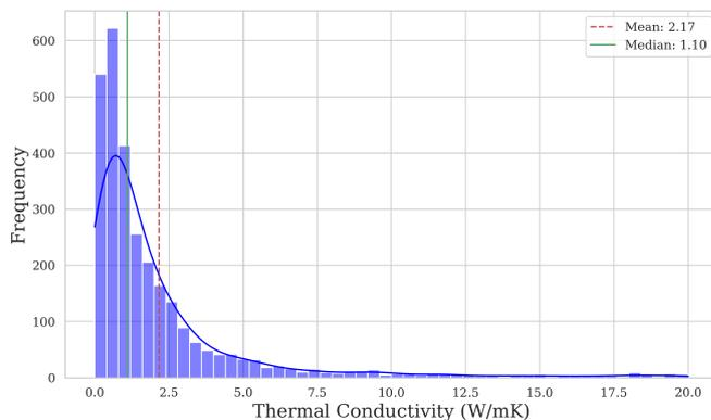
Figure 5: Distribution of Thermal Conductivity in Database
