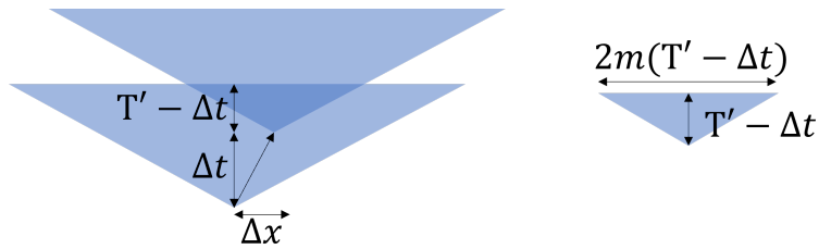
Figure 24: Left: cloning the triangle to find the volume of realisation. Right: the volume of realisation, where the base length is found using similar triangles.
