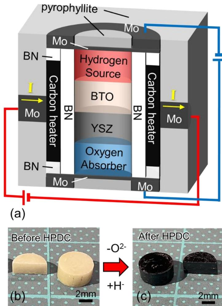
Figure 1. (a) schematic illustration of HPDC. Optical images of BTO (b) before and (c) after treatment.
