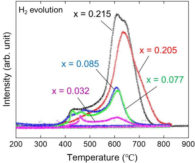
Figure 2. TPD-MS measurements for  $\text{BaTiO}_{3-x}\text{H}_x$ .
