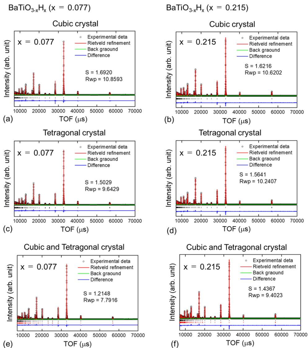
Figure S7. Rietveld refinement analyses of BaTiO<sub>3-x</sub>H<sub>x</sub> (x = 0.077 and 0.215) assuming (a, b) cubic phase, (c, d) tetragonal phase, and (e, f) their mixing phases.
