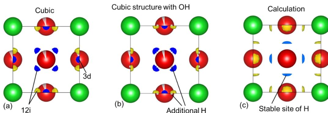
Figure S8. (a) MEM analysis assuming cubic structure. The negative scattering densities are indicated by yellow and blue. (b) MEM analysis assuming cubic structure with OH. (c) DFT calculation for the stable hydrogen position.
