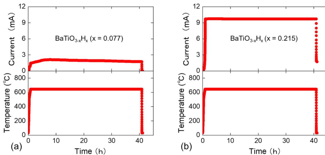
Figure S1. Treatment conditions of HPDC for (a)  $\text{BaTiO}_{3-x}\text{H}_x$  ( $x=0.077$ ) and (b)  $\text{BaTiO}_{3-x}\text{H}_x$  ( $x=0.215$ ).
