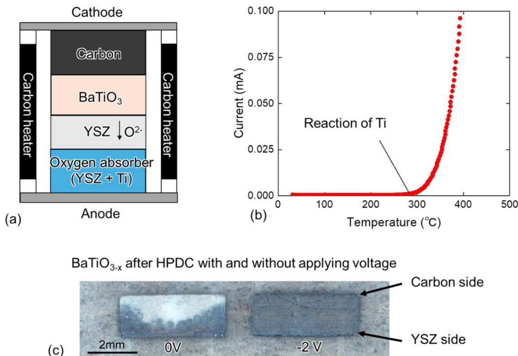
Figure S3. (a) The schematic illustration of sample space to investigate the oxygen extraction by Ti. (b) Temperature dependence of current passed sample space during the HPDC treatment. (c) The cross sections of optical images for the samples after HPDC treatment with and without voltage application.
