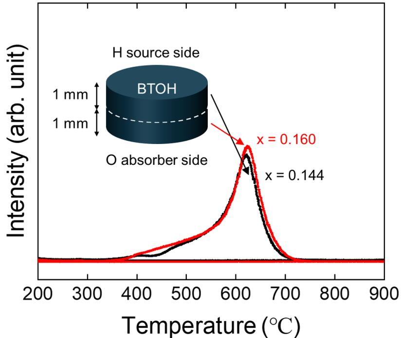
Figure S5. TPD-MS measurements for the upper and lower parts of the sample.
