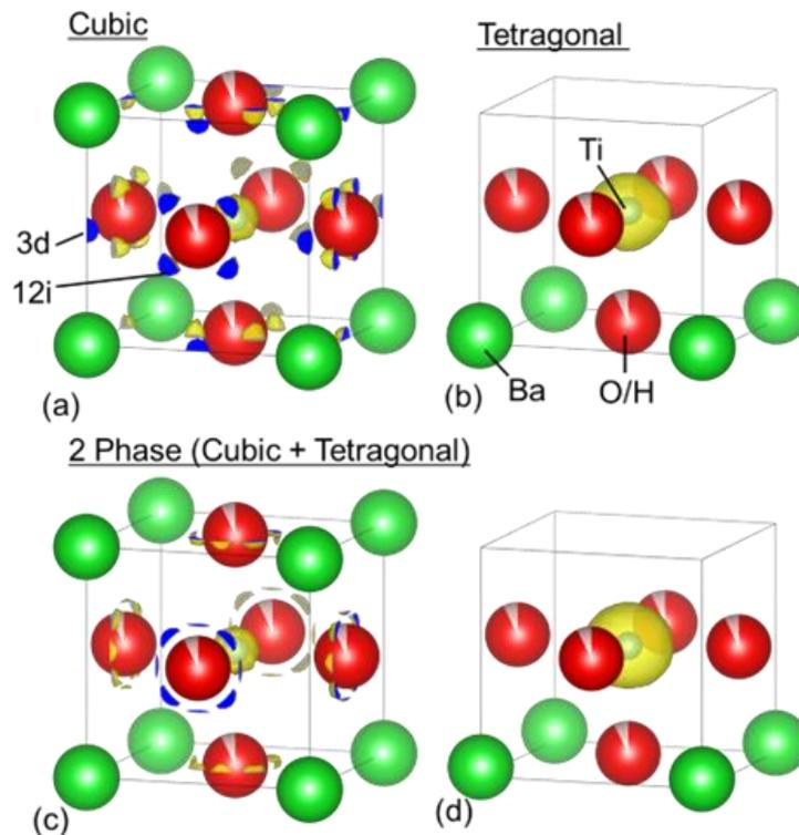
Figure 4. MEM analysis from neutron diffraction measurements of  $\text{BaTiO}_{3-x}\text{H}_x$  ( $x=0.215$ ) assuming (a) cubic, (b) tetragonal, and their mixed phases: (c) cubic and (d) tetragonal. The crystal structures were drawn using the visualization for electronic and structural analysis (VESTA).<sup>30</sup>
