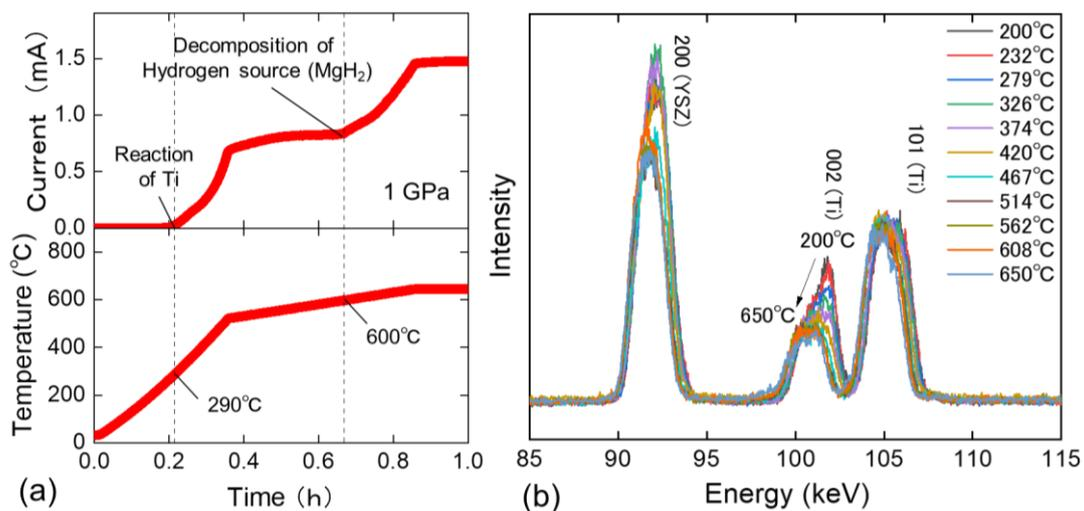
Figure S2. (a) Time and temperature dependence of current passed the sample space at 1 GPa. (b) In-situ observation of oxygen absorber using synchrotron x-ray diffraction from 200°C to 650°C under 1 GPa.
