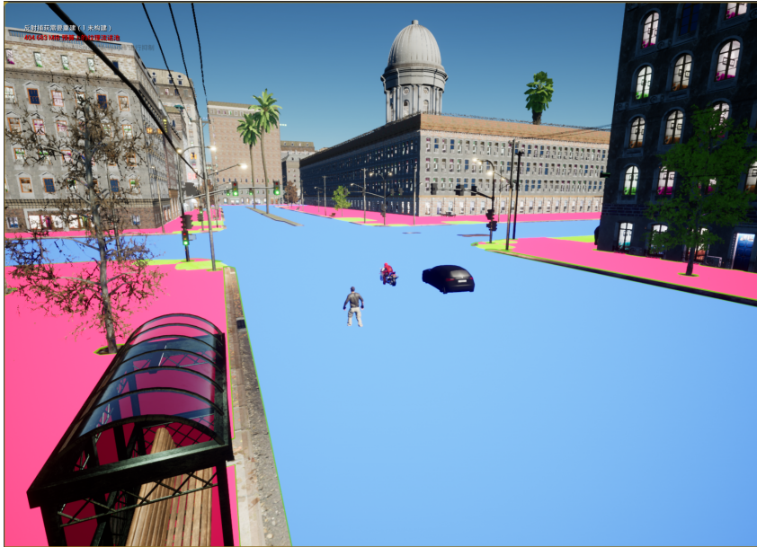
Figure 10: An example of the NavMesh with semantic segmentation. The human character will prioritize using the pink area for pedestrian navigation tasks, while the vehicles will use the blue area.
