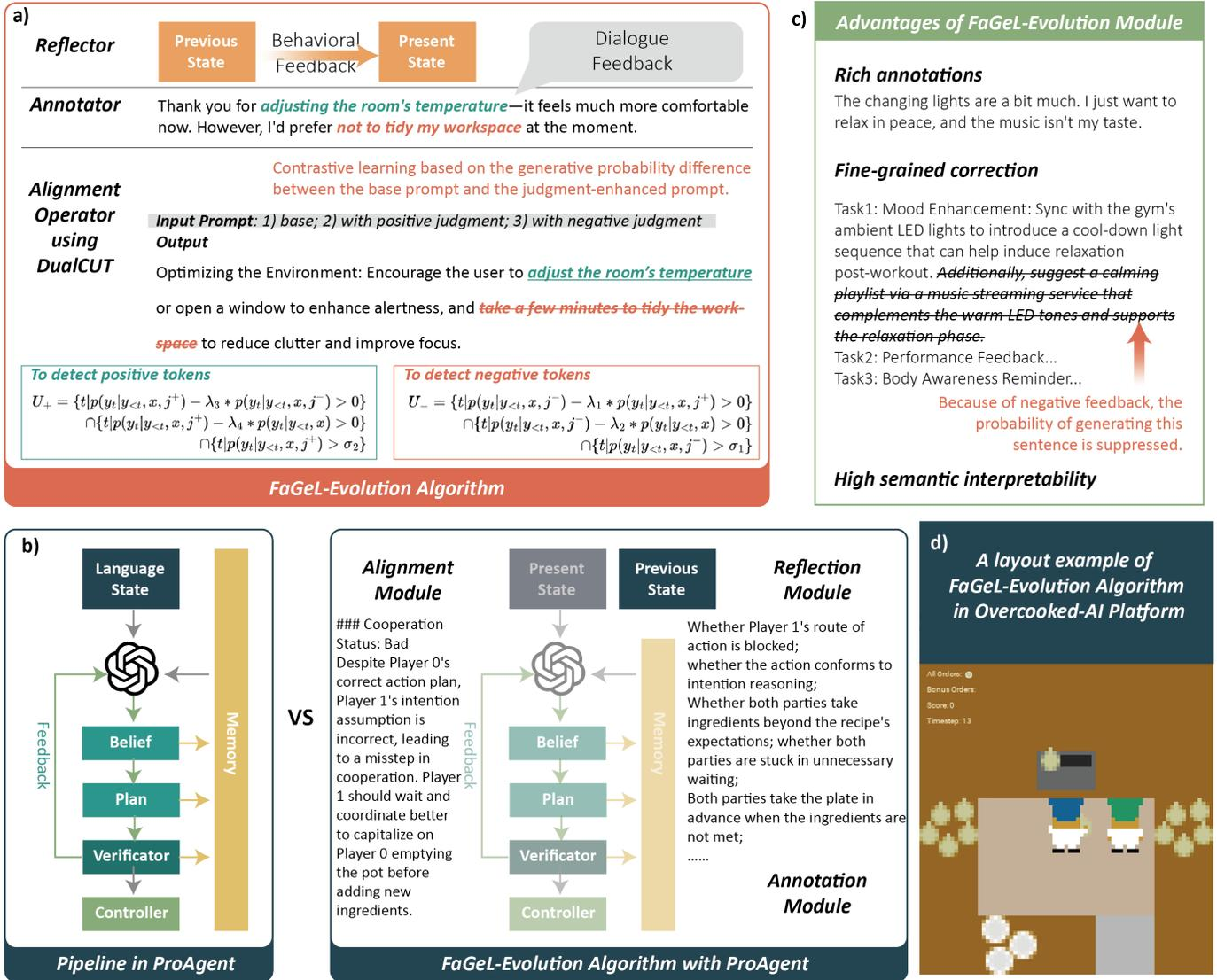
Fig. 2. **Architecture and Implementation of the Intelligence Evolution Module:**(a) Functional components of FaGeL evolution algorithm; (b) The comparison of ProAgent algorithm and FaGeL evolution algorithm; (c) The advantages illustration of FaGeL; (d) Demonstration of the FaGeL evolution algorithm outperforming ProAgent using the Overcooked-AI platform.
