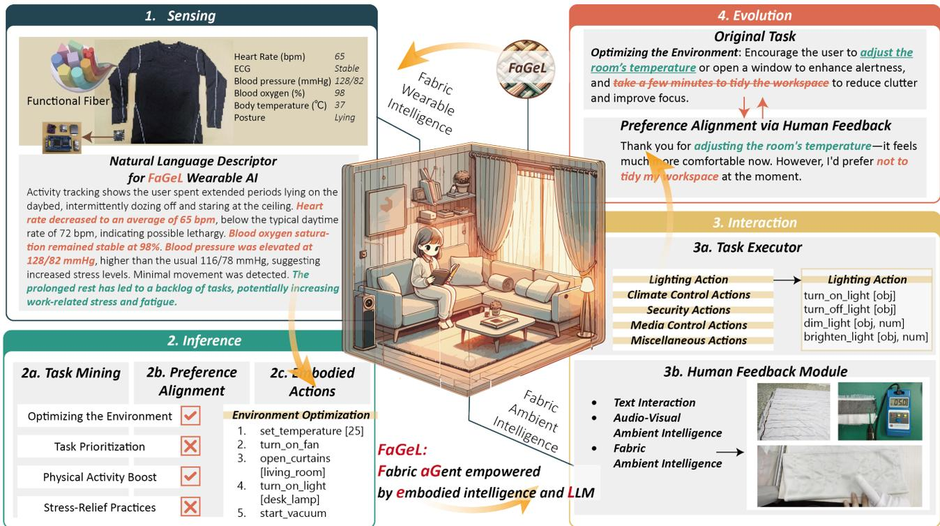
Fig. 1. The Fabric Agent Empowered by Embodied Intelligence with LLM (FaGeL) integrates (1) a sensing module empowered by wearable intelligence, equipped with a natural language descriptor; (2) an inference module composed of task mining, AI alignment, and embodied action decomposition; (3) an interaction module consisting of task execution and user feedback perception; (4) an embodied intelligence evolution module based on token-level AI alignment.
