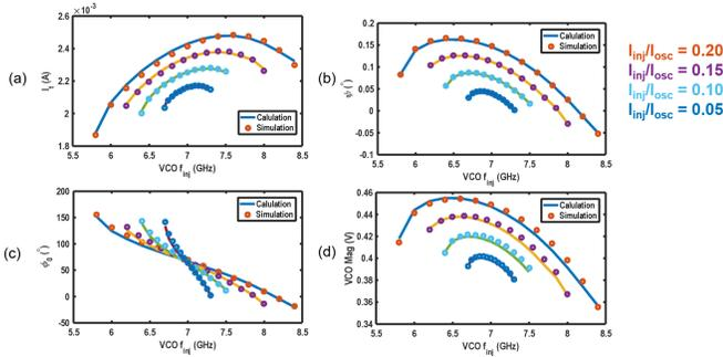
Fig. 14: Calculated and simulated  $I_t, \psi, \phi_0, V_{osc}$  versus injection frequency under injection strength: (a) 0.2; (b) 0.15; (c) 0.10; (d) 0.05.
