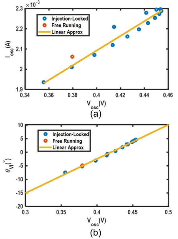
Fig. 7: The amplitude and phase of  $I_{osc}$  in the RO with multi-phase injection enabled and disabled.
