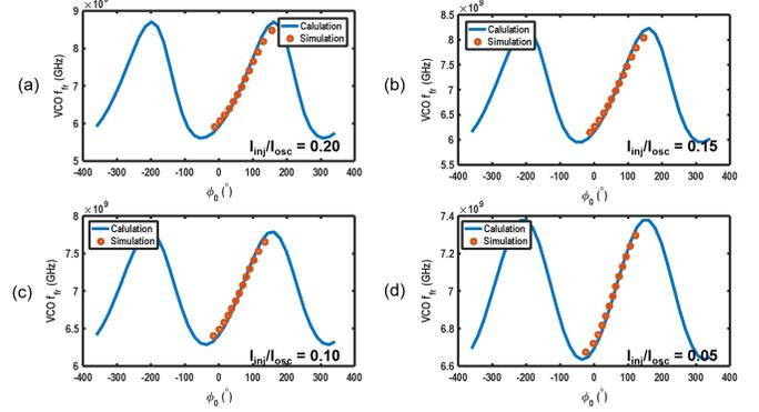
Fig. 11: Calculated and simulated  $\phi_0$  versus free-running frequency under injection strength: (a) 0.2; (b) 0.15; (c) 0.10; (d) 0.05.
