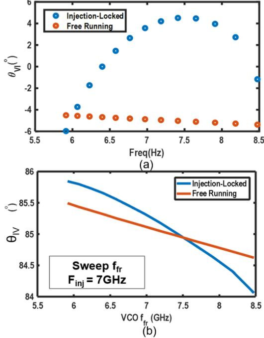
Fig. 5:  $\theta_{IV}$  and  $\theta_{VI}$  versus the free-running frequency of a ring oscillator with multi-phase injection enabled and disabled.
