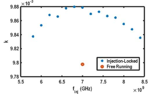
Fig. 8:  $k$  versus different injection frequencies.
