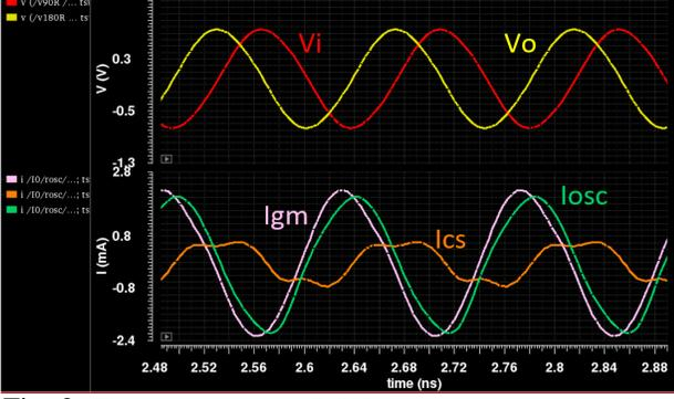
Fig. 2: The waveform of a 7-GHz free-running ring oscillator.
