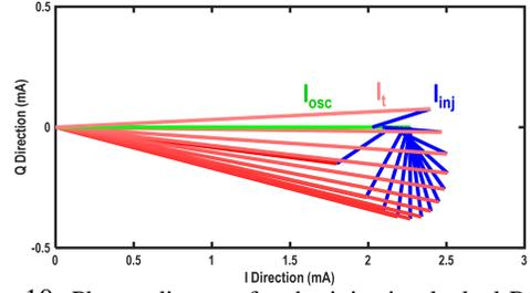
Fig. 10: Phasor diagram for the injection-locked RO with amplitude-to-phase conversion.
