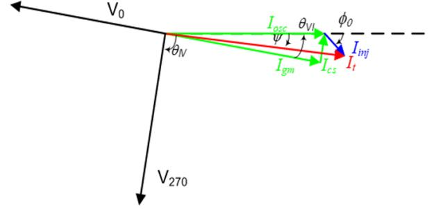
Fig. 4: The phasor diagram of the voltages and currents in an injection-locked ring oscillator.
