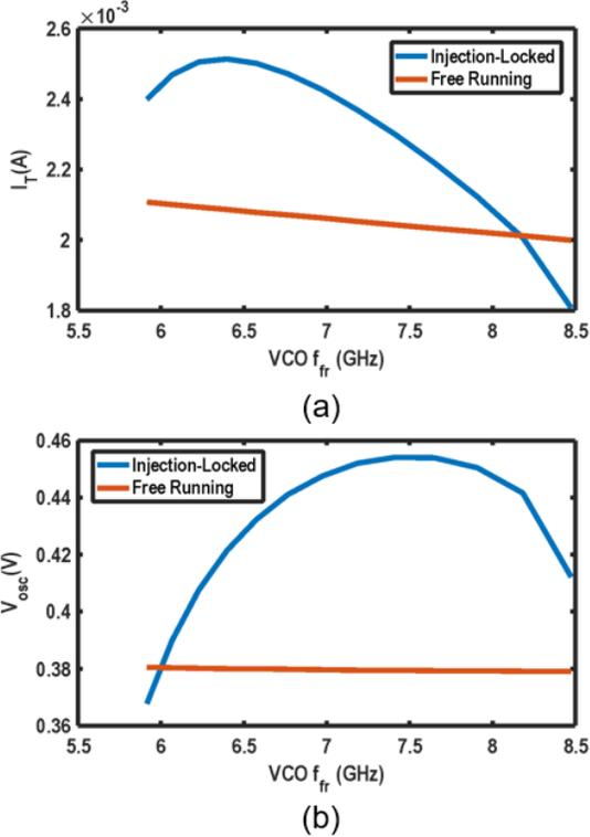
Fig. 6: the phasor amplitude  $I_t$  and  $V_{osc}$  in the RO with multi-phase injection enabled and disabled.
