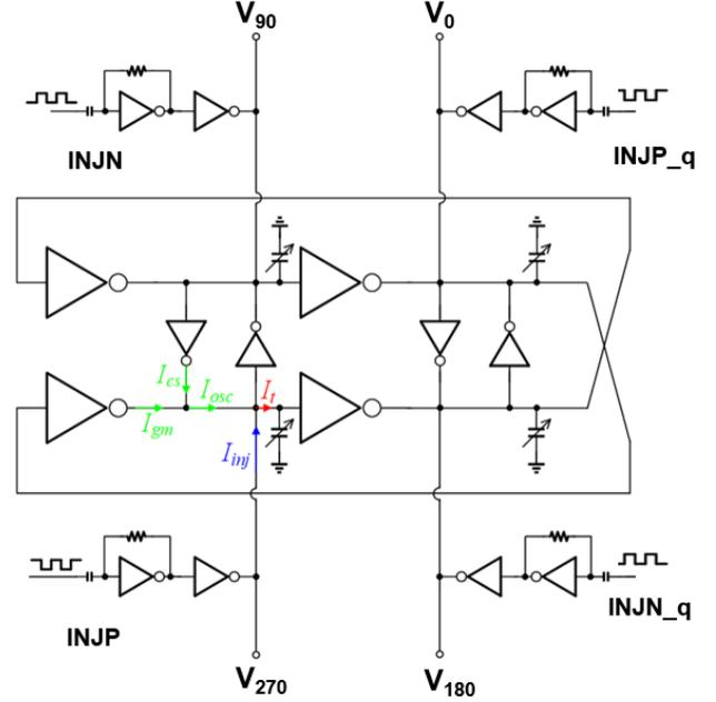
Fig. 1: The schematic diagram of an injection-locked ring oscillator with multi-phase injection.
