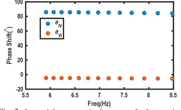
Fig. 3:  $\theta_{IV}$  and  $\theta_{VI}$  versus the frequency of a free-running ring oscillator.
