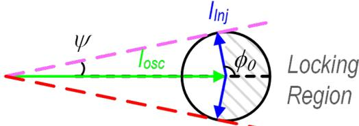
Fig. 9: Phasor diagram for Adler's equation.
