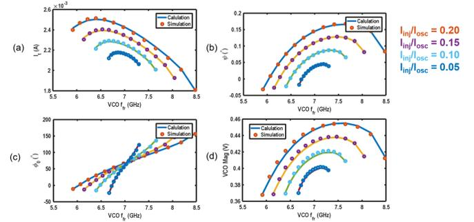
Fig. 12: Calculated and simulated  $I_t, \psi, \phi_0, V_{osc}$  versus free-running frequency under injection strength: (a) 0.2; (b) 0.15; (c) 0.10; (d) 0.05.
