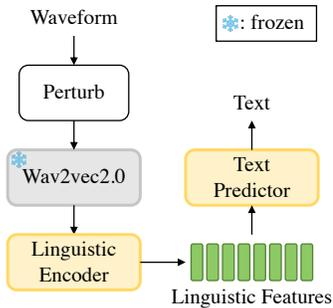
Fig. 4. A pipeline for extracting the target linguistic features from waveform. To eliminate speaker-related features, the perturbed waveform is input to a multilingual wav2vec2.0. The following linguistic encoder extracts solely linguistic features, which are fed into a text predictor.
