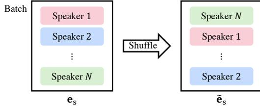
Fig. 3. Batch-wise shuffle operation.  $\mathbf{e}_s$  is the speaker embeddings and  $\tilde{\mathbf{e}}_s$  denotes the shuffled speaker embeddings.
