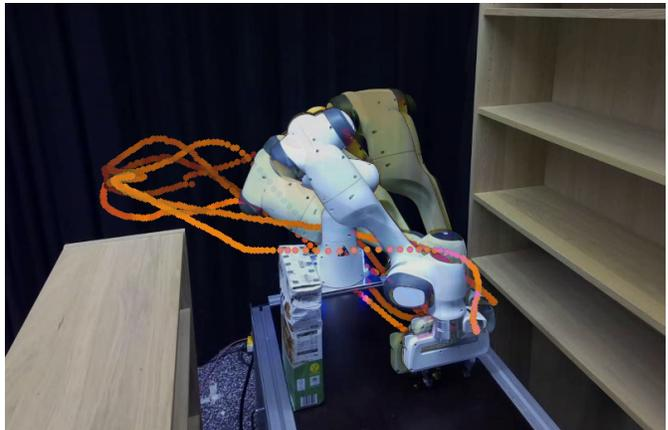
Fig. 9. Example of multimodal trajectories executed in the warehouse environment using MPD. Starting from the same joint configuration, the task is to reach an end-effector pose on the table while avoiding collisions with the environment. The orange lines depict the end-effector trajectories, and the overlaid images show the last frame on the trajectory. Our model generates multiple goal robot configurations for similar desired end-effector poses.
