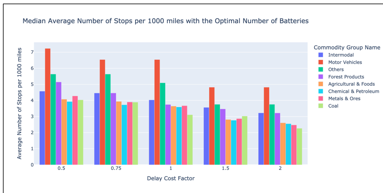
Figure 12 - Median Average Number of Stops per 1,000 miles with the Optimal Number of Batteries under Different Delay Cost Factors
