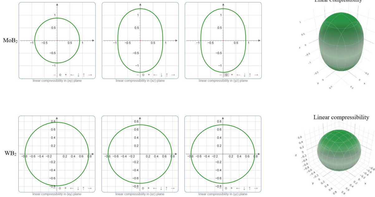
Figure 3. 2D (left) and 3D (right) directional dependences in compressibility ( \beta ) of \text{XB}_2 compounds.
