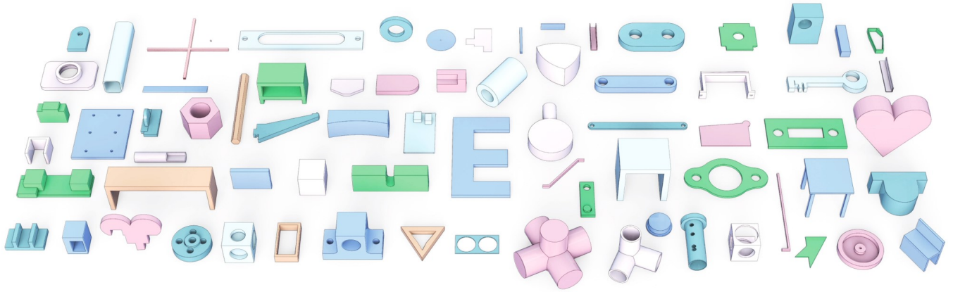
Figure 1: Demonstration of various CAD models generated by CAD-GPT. The models in the image demonstrate semantic sketch generation capabilities (e.g., a heart shape and the letter "E"), category-based CAD generation capabilities (e.g., a table, a chair, and a key), spatial reasoning abilities (e.g., a table and mutually perpendicular cylinders), and the capability to generate identical models with varying dimensions (e.g., three connectors with two circular holes of differing sizes).
