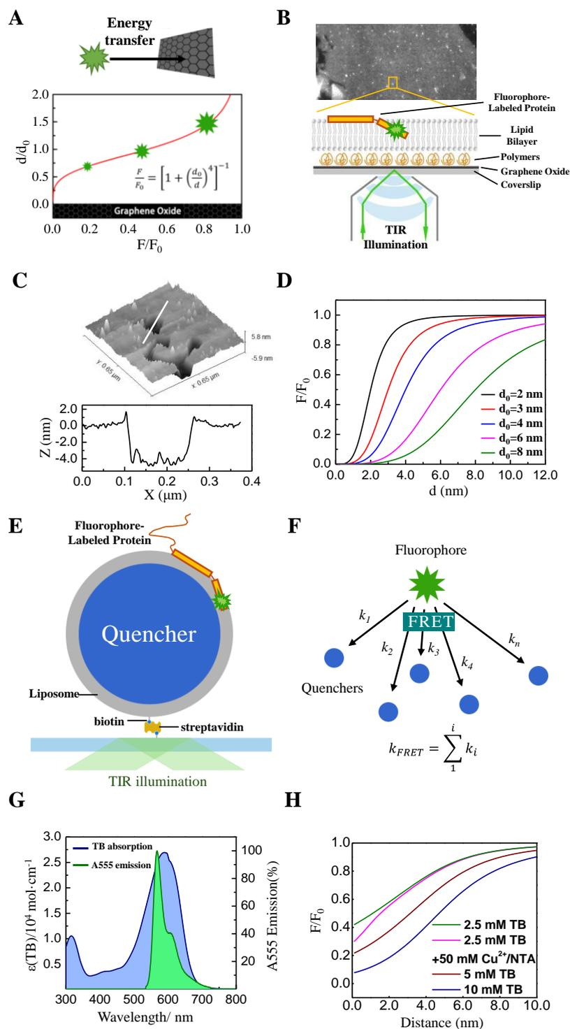
Fig. 1 The principle of SIFA and LipoFRET. (A) The fluorescence of a fluorophore changes rapidly with its distance to a graphene oxide layer. (B) The experimental setup of SIFA on TIRF microscopy. (C) The morphology (upper panel) and the profile of the
