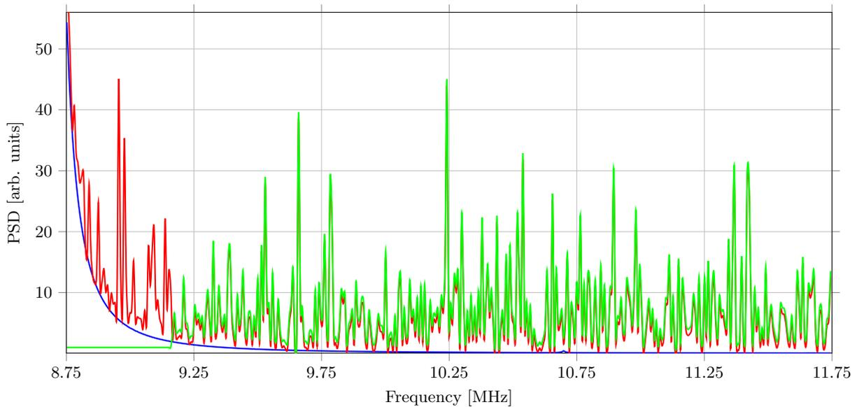
FIG. 3: Comparison of the simulated signal spectrum (blue), noisy spectrum (red), and the spectrum after excluding the longitudinal signal component (green). The spectrum is simulated at a revolution frequency of 6.4 MHz to illustrate the exclusion of the longitudinal signal component. Typical SAPT values, as in Fig. 2, are assumed.
