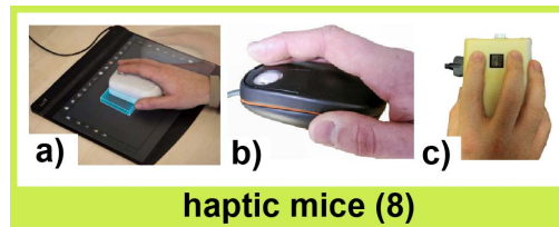
Fig. 13. Examples of haptic mice: a) a haptic mouse that assists people with BLV in comprehending 3D shapes for their O&M education [28]; b) ViPong: a haptic mouse to assist people with BLV in playing games [234]; c) a haptic mouse that assists people with BLV in understanding graphics with different details [185].
