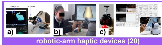
Fig. 9. Examples of robotic-arm haptic devices: a) a multimodal robotic-arm haptic device that assists people with BLV to build 3D models independently [141]; b) A robotic-arm haptic device that assists people with BLV’s education. The figure shows how it supports the students with BLV in comprehending various shapes [63]; c) A robot and robotic arm system to assist people with BLV in telepresence [185].
