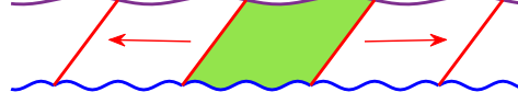
Figure 4: A 1D lattice with two boundaries and the unit cell domain with single periodic boundary.
