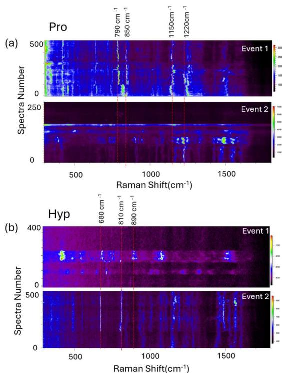
Figure 2. Waterfall plot of typical Raman spectra of (a)proline and (b)hydroxyproline trapping event. The color bars indicate the signal-to-base peak intensity.
