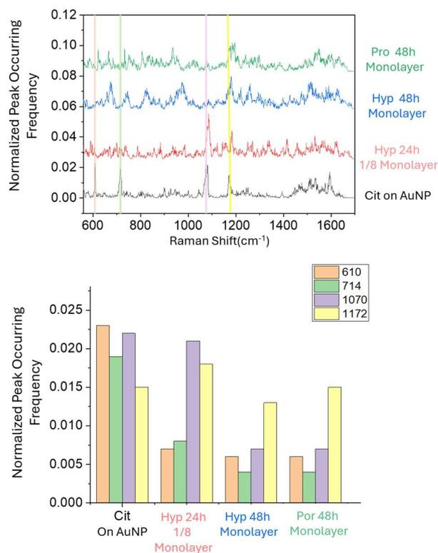
Figure 4. (a) The normalized peak occurring frequency generated in particle-in-pore sensors using AuNP with citrate capping (black curve), 24h incubation in solution with Hyp concentration for 1/8 monolayer (red curve), 48h incubation in solution with Hyp concentration for a monolayer (blue curve), 48h incubation in solution with Pro concentration for a monolayer. Four characteristic peaks of citrate-capped
