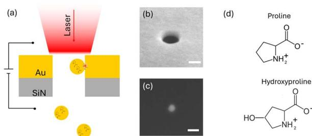
Figure 1. (a) Schematic illustration of the particle-in-pore sensor that allows single AuNPs loaded with analytes to be trapped in a gold nanopore with plasmonic resonance upon laser excitation at 785 nm. (b) SEM image of the nanopore. The scale bar is 200nm. (c) SEM image of the AuNP. The scale bar is 100nm. (d) The molecule structure of proline and hydroxyproline at pH5.5 in solution.
