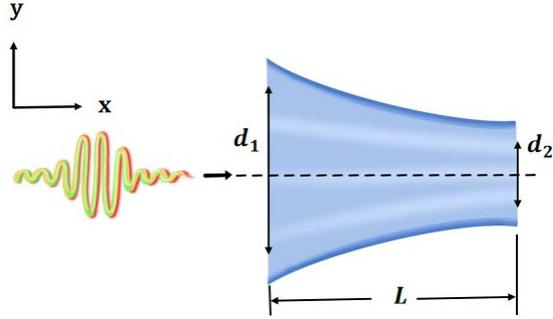
FIG. 1: The schematic diagram of an attosecond electron bunches generated by the interaction of an ultra-intense laser with a gold curved wall conical channel and the geometry of the curve wall is hyperbola. The parameters of the conical channel are:  $d_1 = 10\mu\text{m}$ ,  $d_2 = 5\mu\text{m}$  and  $L = 25\mu\text{m}$ .
