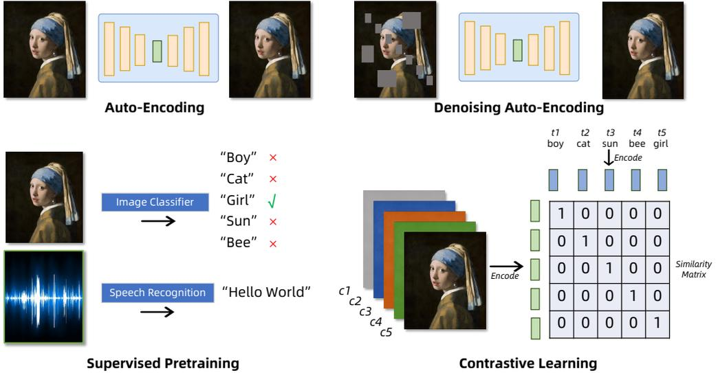
Fig. 5. Illustrations of the training method of tokenizers.
