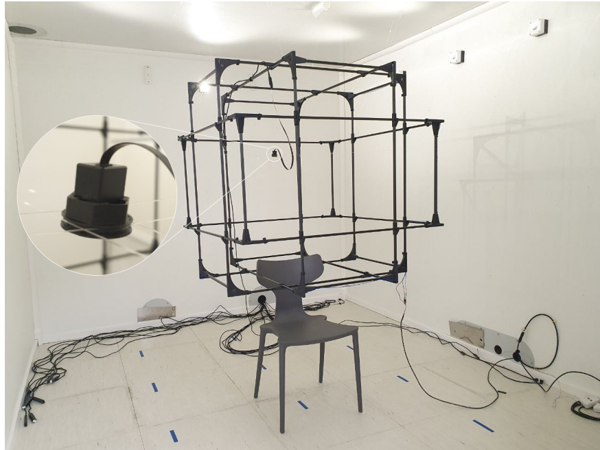
Figure 3: DASS’s coils installed in room 2. Each pair of Helmholtz coils comprises square coils of dimension 1\text{ m} \times 1\text{ m} located 0.5\text{ m} apart and positioned in the three orthogonal planes. The QuSpin Gen-2 OPM, that is the internal reference sensor, is shown in the inset.
