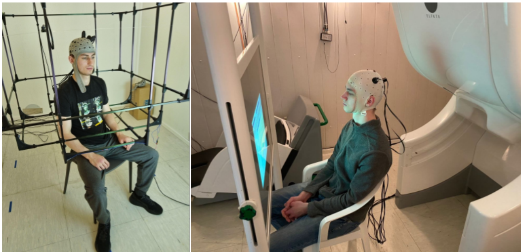
Figure 4: Participants in the two experimental environments: MEG Center MSR (right) and HSE MSR (left). The coil of the digital adaptive suppression system in the HSE room is also visible.
