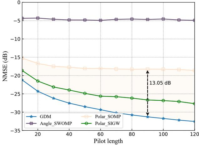
Fig. 2. NMSE performance of CSI acquisition utilizing GDM.
