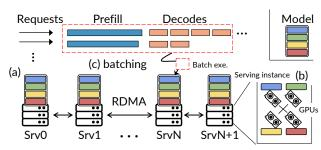
**Figure 2:** An illustration of a typical LLM serving scenario (a): how the model is deployed on each server with different serving instances (b) and (c) how prefill and decode requests are processed in a batched way. *exe.* is abbreviated for execution.
