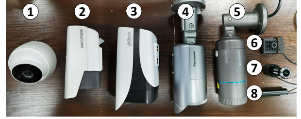
Figure 16. The 8 commercial analog cameras tested in the evaluation: ① HIKVISION DS-2CE56C3T-IT3 [60], ② HIKVISION DS-2CE16G0T-IT3 [53], ③ DH-HAC-HFW1200M-I2 [61], ④ Panasonic WV-CW314LCH [62], ⑤ SAMSUNG SCO-2080RP [63], ⑥ SONY CCD673-1200, ⑦ SONY CCD-1200, and ⑧ SONY IMX323 [64].
