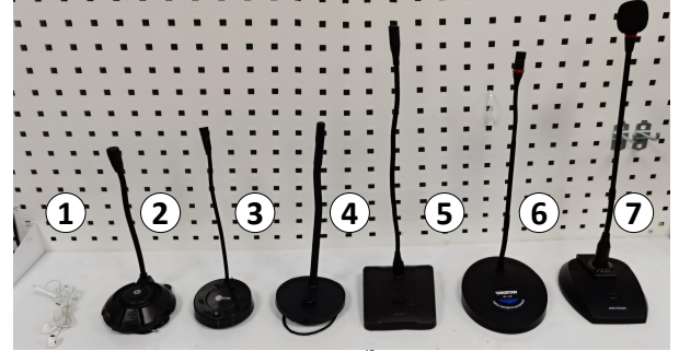
Figure 17. The 7 commercial microphones tested for evaluation: ① wired earphone HUAWEI AM115 [65], ② desktop microphone HP DHP-1100I [66], ③ desktop wired microphone Lenovo Lecoo MC01 [67], ④ USB microphone UGREEN CM564 [68], ⑤ broadcast microphone SM88, ⑥ conference microphone TAKSTAR MS-118 [54], ⑦ conference microphone HIKVISION DS-KAU30HG-M [69].
