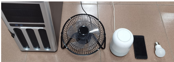
Figure 20. We evaluate the impact of electrical noises on PowerRadio by plugging 5 typical IoT devices into the household power system.
