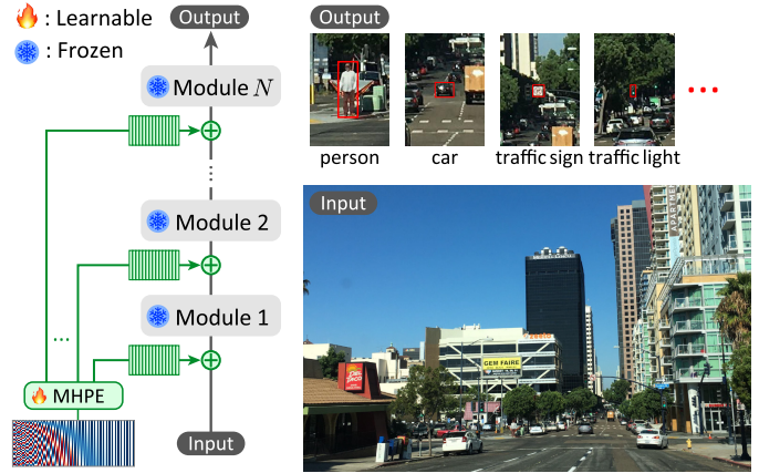
Fig. 1. Multi-point positional insertion (MPI) tuning for small object detection. MPI tuning inserts positional embeddings at multiple points in a frozen pretrained model through a learnable multi-head positional encoder (MHPE). This figure illustrates a frozen object detection model with N sequential modules for simplicity.
