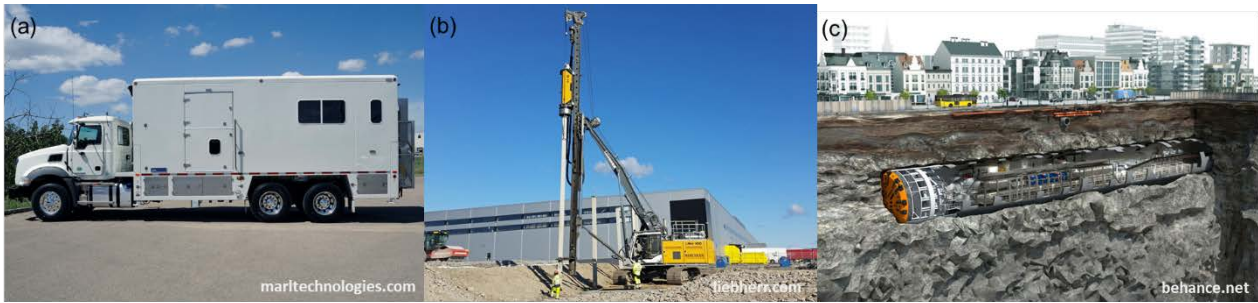
Figure 1. Geotechnical equipment for soil penetration and excavation: (a) rig for CPT and DMT testing, (b) hammer for pile driving, and (c) boring machine for tunnel construction.
