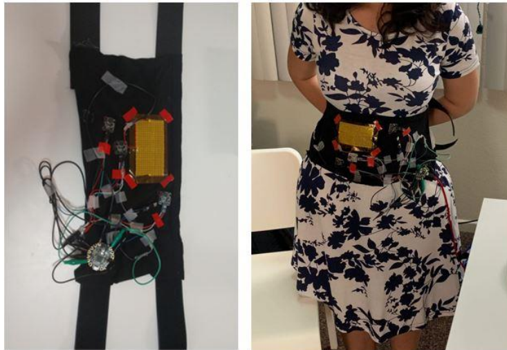
Figure 8: The belt with the vibration motors and Flora
